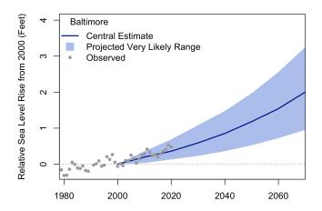
The graph shows the projected change of sea level in feet above mean sea level relative to 2000. The blue line shows the intermediate scenario (50% probability) and the blue shading shows the low to high scenario range (5 to 95% probability) of sea level rise used for official planning purposes in Maryland. Dots show the observed changes in sea level at sIrname tide station. Data for the future scenarios are based on a low-emissions scenario (RCP 4.5).
