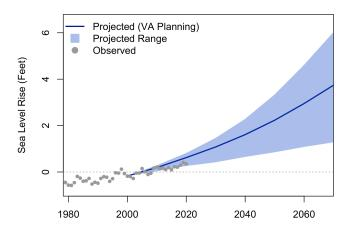
The graph shows the projected change of sea level in feet above NAVD88 compared to the 1983-2001 average. The blue line shows the sea level rise scenario used for official planning purposes in Virginia. The blue shading shows the range between the low and extreme scenarios for sea level rise. Dots show the observed changes in sea level at Sewell's Point, VA.
